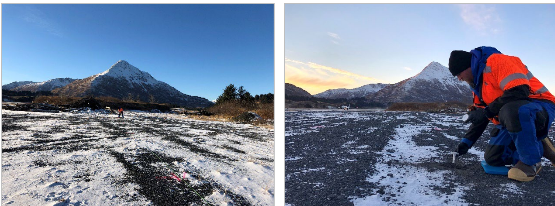
Exhibit 2-4: Field staff mark decision unit boundaries at ADQ-ISM1 (left), and field staff use a Terra Core® sampler to collect a sample increment of soil for GRO and VOC analysis from ADQ-ISM1.
